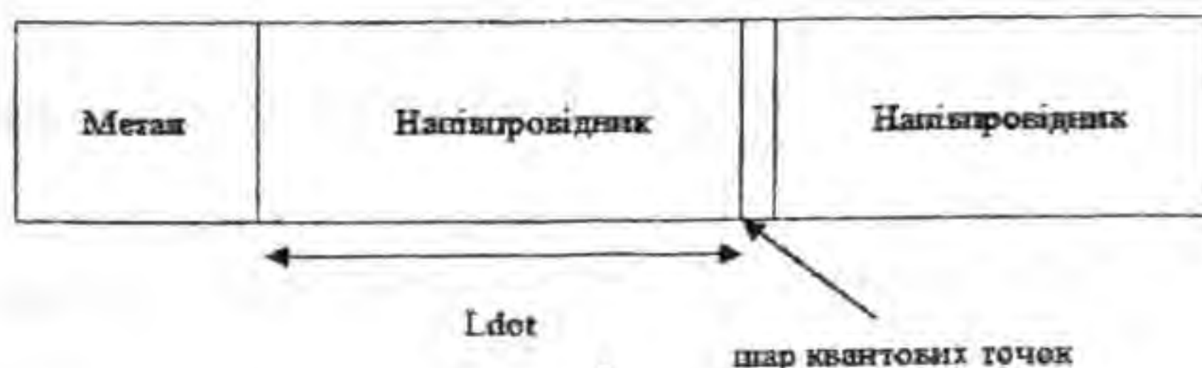
Fig.1. Metal-semiconductor contact with embedded QD layer
