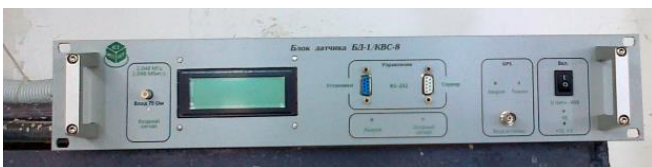
Fig. 6. Block of sensors SB-1 of the control and measurement system of the quality of synchronization signals (CMS-8)
