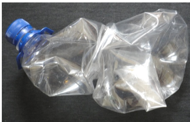
Fig. 1. A closed polyethylene bottle with hydrogen gas after 2 weeks of filling. These changes shows that hydrogen gas easily can permeate through the polyethylene.
